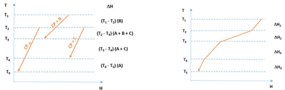
In the graph above, the three hot streams are plotted separately, with their supply and target temperatures defining a series of "interval" temperatures  $T_1$ - $T_5$ . Between  $T_1$  and  $T_2$ , only stream B exists, and so the heat available in this interval is given by  $B \times (T_1 - T_2)$ .
